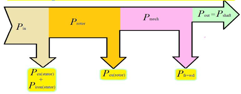
$$P_{in} = P_{rotor} + P_{cu(stator)} + P_{iron(stator)}$$
