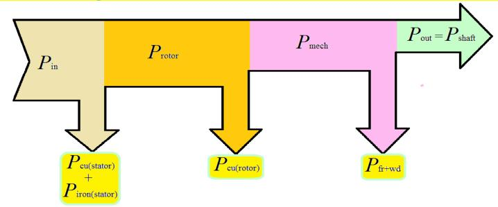
$P_{\rm in}$  input power to the motor or to the stator (Watt)
